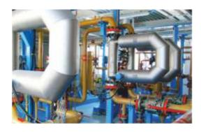
**Measurement Systems** are designed for automated quantity accounting crude, marketable oil or petroleum products indirect bulk or direct mass dynamic method according recommendations No. 69 of March 31, 2005, GOST R 8.595, MI 2825, GOST R 8.615, MI 2693.
